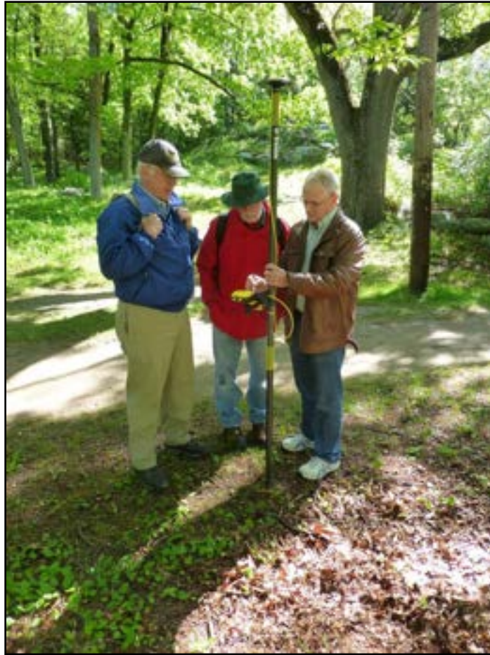
Figure 37 Site surface survey with Trimble GeoXT and GeoXH series 6000 GPS. (From the left: Rose, Poole, and Griswold.)
