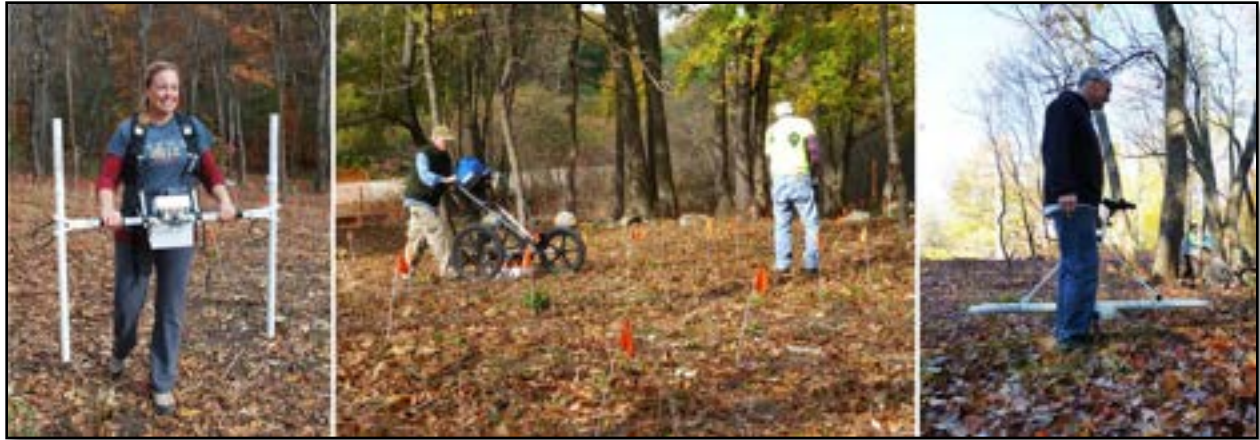
Figure 41 Geophysical survey equipment and pin flag grid. Bartington Grad601 fluxgate gradiometer (Watters), GSSI ground penetrating radar (Rose with Poole on flags), and the GSSI Profiler conductivity (Griswold).
