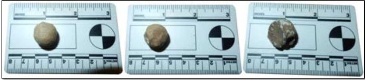
Figure 94 British fired musket balls: low (FS33A), medium (FS2A), and high (FS22A) velocity impact.
